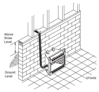
Figure 12 -Basement Installation
