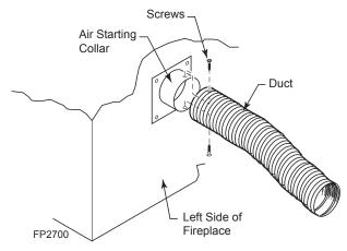
Figure 17 - Attach Outside Duct to Starting Collar
