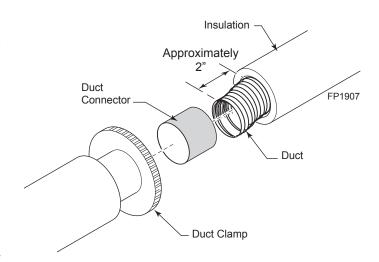
Figure 19 -Install Duct Connector 403
