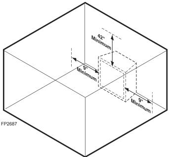
Figure 4 - Clearance and Height Requirements
