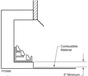
Figure 7 -Minimum Clearance Above Combustible Flooring
