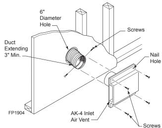
Figure 18 -Combustion Air Assembly for Model AK-4
