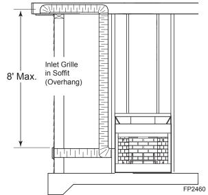
Figure 13 -Concrete Slab Installation (Optional Outside Air Runs)
