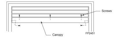
Figure 11 - Installing Canopy
