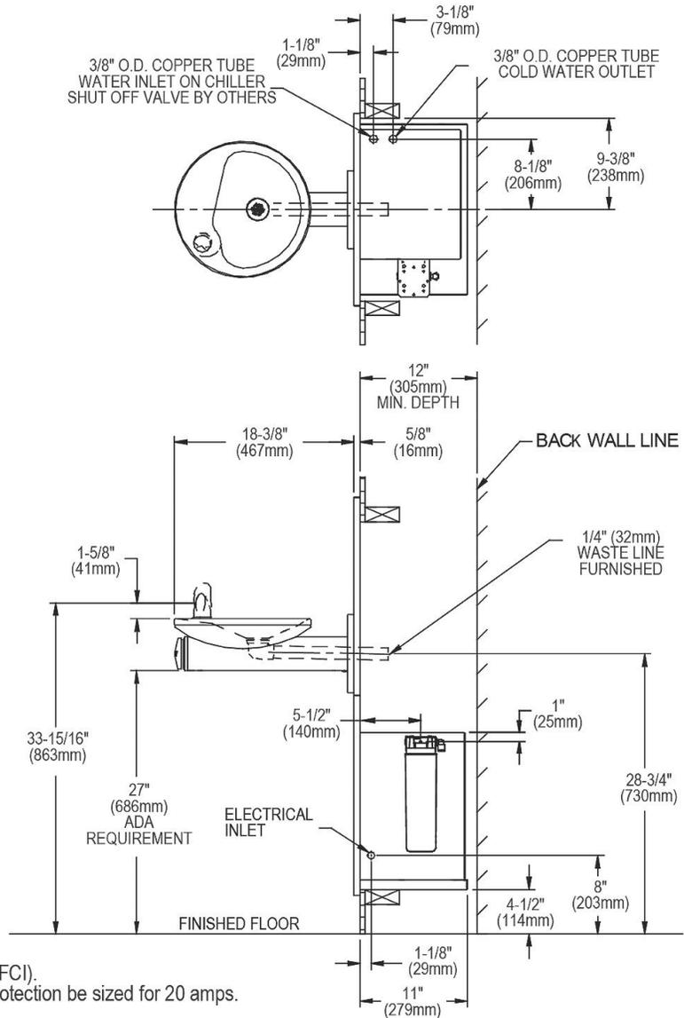
Note : New Installations Must Use Ground Fault Circuit Interrupter (GFCI).
