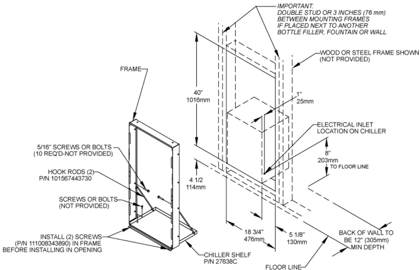
1. **Cut a square rectangular wall opening** 18 3/4" (476mm) W x 40" (1016mm) H and 4 1/2" (114mm) above the floor line.
