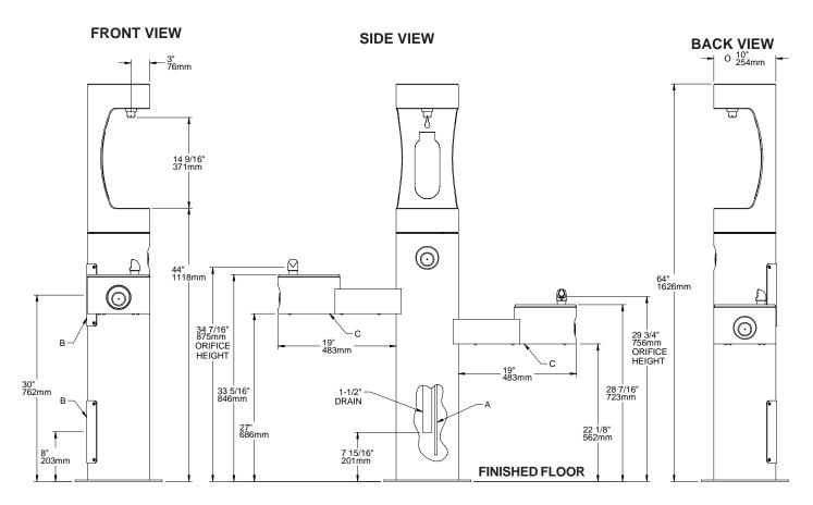
LEGEND A = 3/8" O.D. UNPLATED COPPER TUBE CONNECT - SHUT OFF VALVE BY OTHERS B = ACCESS PANEL (8" X 10") C = REMOVABLE BOTTOM COVER
