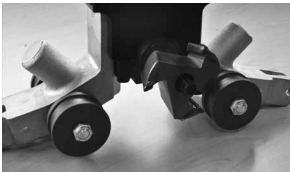
3. Tighten PVC Bevel Cutter onto Long Arbor
