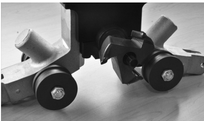
3. Tighten PVC Bevel Cutter onto Long Arbor
