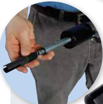
FTPSAA & PL688 attaching to coupling nut
