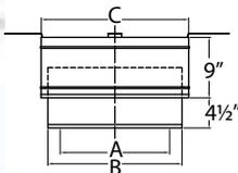
Supports chimney pipe and provides a positive connection between support box and chimney. Supports up to 40' of DuraTech Chimney. Trim collars are sold separately. (For 10" use DuraBlack Slip Connector to attach DuraBlack to the support box. See DVL/DuraBlack section).
