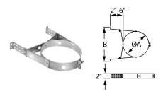
Use in interior or exterior installations to support and to stabilize the chimney while assuring a 2" clearance. Wall straps are required every 4' on exterior of building. Adjusts 2"-6" from wall.
