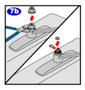
Using pliers, loosen and remove the pivot retainer nut as well. Remove the washer from the cartridge. Pull the stem up on the old cartridge to relieve any pressure in the faucet then use pliers to remove the retaining clip.
