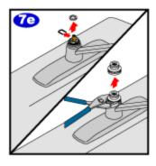
To reinstall the cartridge into your faucet assembly, reverse the steps that you followed to remove the old cartridge. Replace the washer onto the cartridge stem. Using pliers, secure the pivot retainer nut to the faucet assembly.
