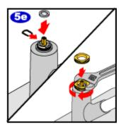
To reinstall the cartridge into your faucet assembly, reverse the steps that you followed to remove the old cartridge. Reinstall the washer onto the cartridge stem and reattach the retainer nut.
