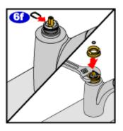
To reinstall the cartridge into your faucet assembly, reverse the steps that you followed to remove the old cartridge. Reinstall the washer onto the cartridge stem and reattach the retainer nut with adjustable pliers.
