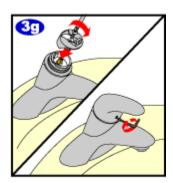
When reattaching the handle, make sure to hook the back of the adapter into the groove of the pivot retainer.
