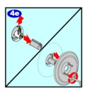
To reinstall the cartridge into your faucet assembly, reverse the steps that you followed to remove the old cartridge. Reinstall the retaining clip, the limit stop and the washer onto the cartridge. Fasten the escutcheon to the wall.
