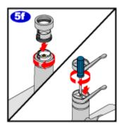
Place the black plastic pivot retainer with 2 grooves facing the back of the faucet on. Tighten the collar on to the faucet assembly. Lastly, reattach the handle and click the handle cover into place. Go to step 8 if you want to reverse the Hot and Cold sides.
