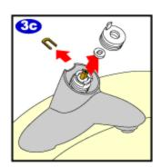
Pull up on the stem of the cartridge to relieve any pressure in the valve.
