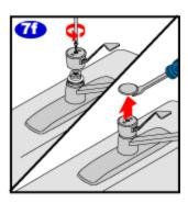
To reattach the handle, align the flat edge of the metal lever under the ridge on the retainer nut, towards the back of the nut. Then bring the handle down in the front so it drops into place. Secure the handle with the screw and snap the handle cover into place. Go to step 8 if you want to reverse the Hot and Cold sides.
