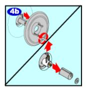
To get access to the cartridge, unscrew and remove the faucet escutcheon. Remove the washer and the limit stop from the cartridge and use pliers to remove the retaining clip.
