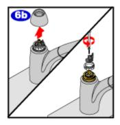
Lift off the decorative dome, unscrew the black plastic pivot retainer, and remove it. Remove the connector screw and lift off the adaptor and connector assembly. Next, remove the white handle stop.
