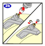
Pull the handle off from the faucet and pull the limit stop off. Remove the washer from the cartridge and use pliers to remove the retaining clip. Pull the stemp up on the old cartridge to relieve any pressure in the faucet.
