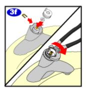
To reinstall the cartridge into your faucet assembly, reverse the steps that you followed to remove the old cartridge. Replace the retaining clip and reinstall the washer and the limit stop onto the top of the cartridge. Replace the collar(s), you would have had 1 or 2 depending on the version of your faucet.
