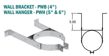
Used to provide lateral support while maintaining proper clearance. Recommended spacing is 6ft. between bands above the starting point.
