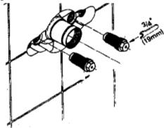
3) Remove Thermo cartridge using a 24mm wrench and clean screen that wraps around the outside of the cartridge and the screen at the backside of the cartridge Cartridge number 47.025.000
