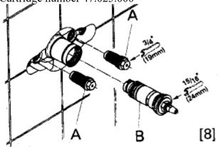
4) Once the thermo cartridge is reinstalled the valve will need to be calibrated, with a thermometer have the water flowing and turn the stem of the cartridge clockwise or counterclockwise until the temperature reaches 100 degrees and is holding, at that time the handle can be installed with the 100 degree marking at 12:00 position.
