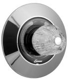
**IMPORTANT:** After completion of installation step 4, follow these instructions to set the Temptrol II Limit Stop Screw. This valve is equipped with a limit stop screw to be used to limit valve handle from being turned to excessively hot water discharge temperatures. To adjust, remove dome cover, open valve to maximum desired temperature and turn in limit stop screw until it seats.
