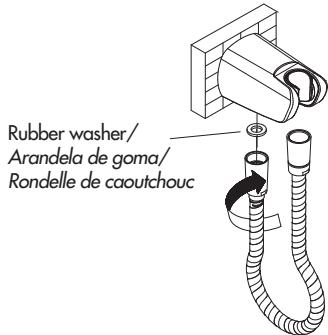
4. Attach one hose conical to the outlet of the supply mount (Danze shower hose will have two flat areas on the hose conical). Use adjustable wrench to tighten the conical if necessary. Note there should be a rubber washer between the outlet and the hose conical.
