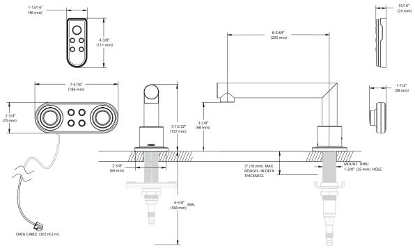
NOTE: THE INSTALLATION SHOWN IS FOR TILE DECKS, THIS VALVE WILL ALSO FIT STEEL, CAST IRON OR PLASTIC DECKS CRITICAL DIMENSIONS
