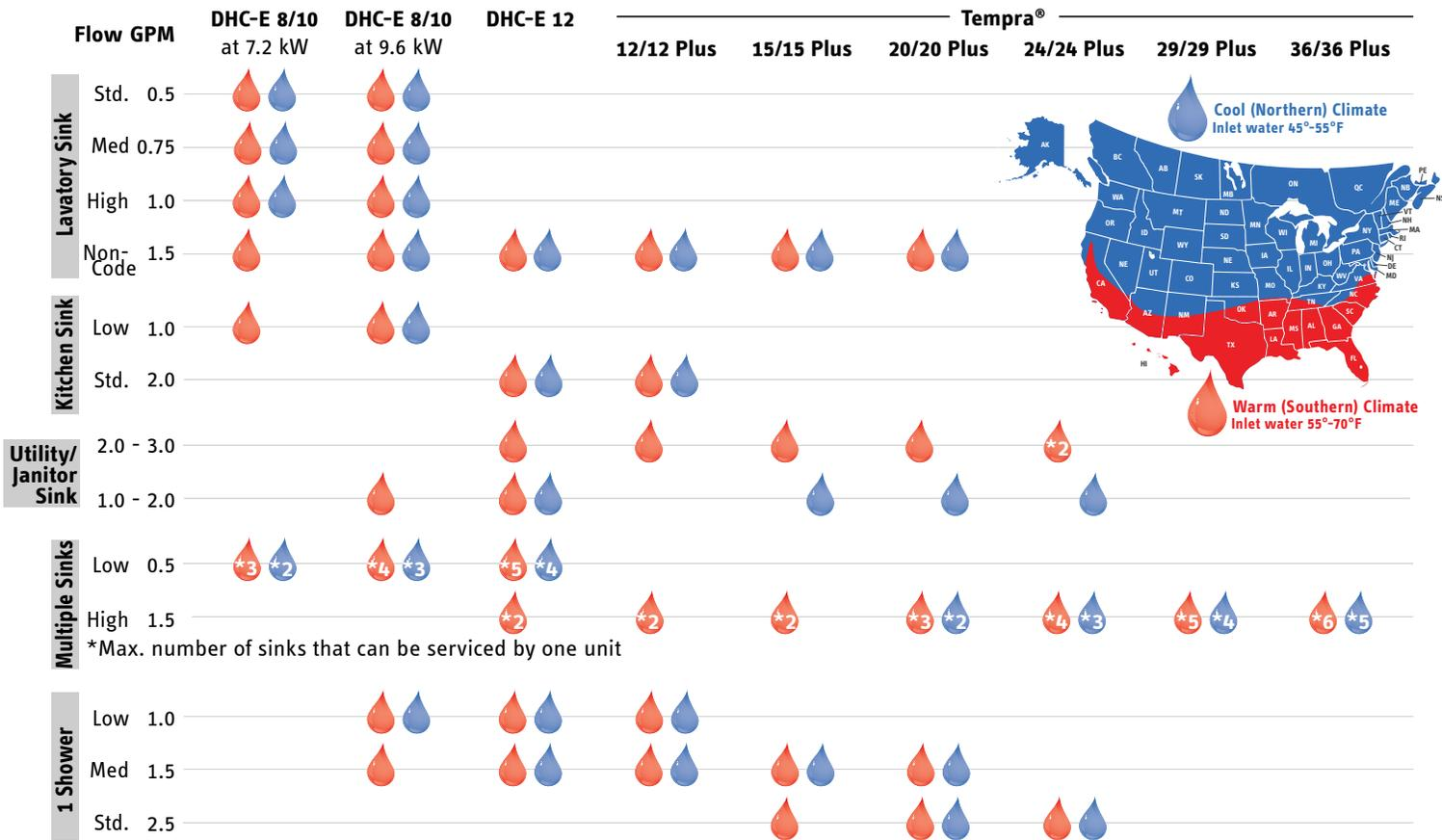
These recommendations are for units installed with 240 V service. Increase one model size if unit will be installed with 208 V service.
