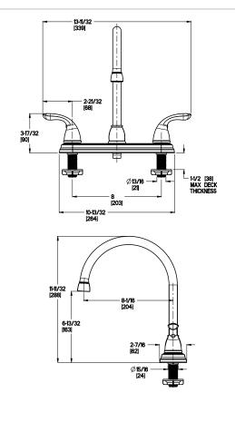
Ø1-3/8 Min to Ø1-1/2 Max. Deck Hole Openings
