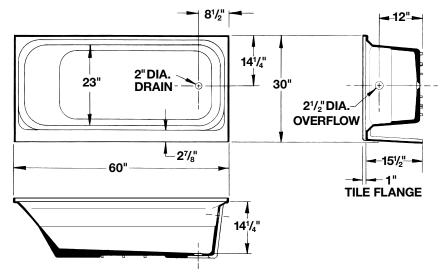
**General:** Furnish and install as shown on plans, TOPAZ<sup>®</sup> bathtub as manufactured by E.L. Mustee & Sons, Inc. Shall be a fiberglass 30" x 60: right hand or left hand Model \_\_\_\_\_\_. Construction shall be molded, reinforced fiberglass using matched metal molds under extreme heat and pressure. Shall meet ANSI Specification Z 124-2011. Color: \_\_\_\_\_\_ (White, Bone, Biscuit) Weight: 74 lbs. Install in compliance with local codes.
