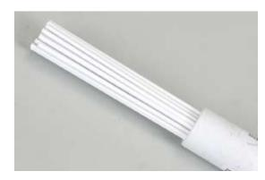
Flux coated, low fuming brazing rod. Provides all properties for best tensile strength and ductility. Rod fuses well with cast iron, malleable iron, galvanized iron, steel, brass and copper. 65,000 PSI tensile strength.
