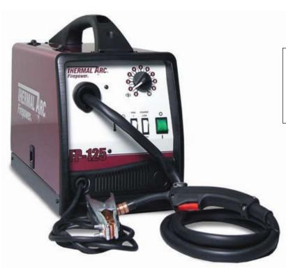
The FP-125 dual-purpose MIG welder offers maximum versatility. The unit features quick-change internal polarity adjustment that makes changing from MIG (GMAW) to flux cored (FCAW) welding quick and easy. With a standard 115 volt household current, it is suitable to use for home projects, but its versatility and 20% duty cycle also makes it ideal for medium duty general repair work and light industrial applications.
