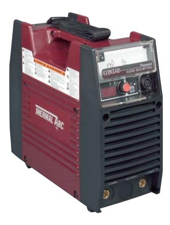
The Thermal Arc ArcMaster 160 S is a multi voltage; full digital control, DC, Stick/Lift TIG inverter power supply. Standard features include: lift TIG start, VRD, adjustable hot start, arc force control and cellulose E6010 compatibility. This is the ultimate compact, highly portable unit designed for Stick and lift TIG welding processes.
