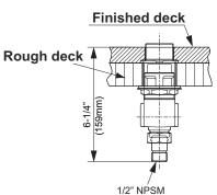
IMPORTANT NOTE: This valve/trim can only be installed in a built-up deck. It cannot be installed on pre-finished deck or on tub rim.
