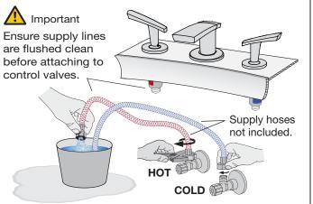
Step 9 Connect supply lines, check for leaks
