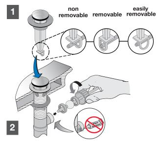
Step 6 Install stopper and pivot rod to drain
