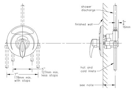
NOTE: 2-1/2" (64mm) min. 3" (76mm) max. On 2"x4" construction, use 2-1/2" (64mm) min. rough-in.
