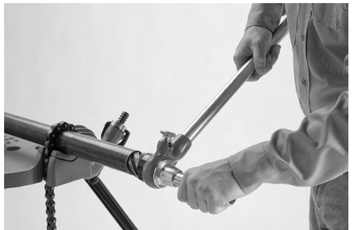
Figure 4 – Reaming End Of Pipe
