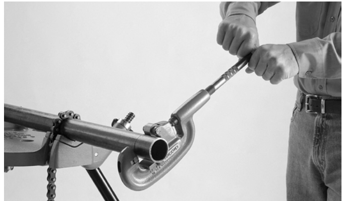
Figure 3 – Cutting End Of Pipe
