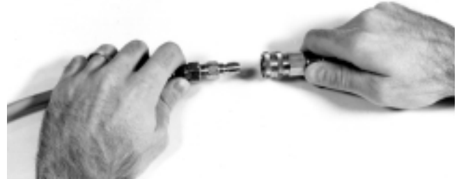
Figure 2 – Connect Jetter Hose
