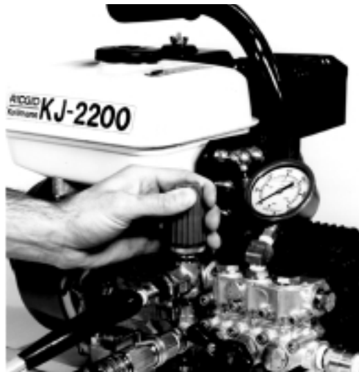
Figure 4 – Adjusting the Unloading Valve
