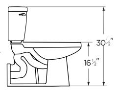
THIS FIXTURE QUALIFIES ACCORDING TO ASME TEST PROCEDURES AS A LOW CONSUMPTION WATER CLOSET WITH AN AVERAGE CONSUMPTION OF 1.6 gpf (6.0 Lpf) OR LESS.
