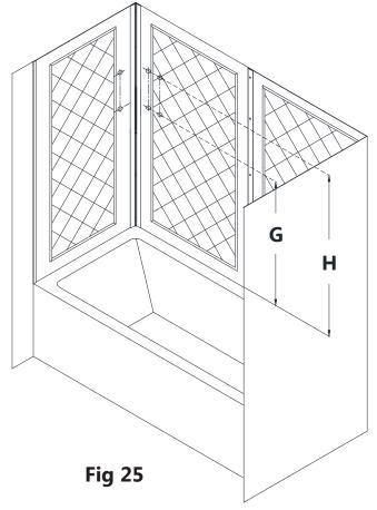
**26.** Mark the location for the **Shelf Brackets (#10)** according to the measurements in <u>Fig 25.1</u>. Drill the holes using **Ø5/16**" drill bit and insert the **Wall Anchors (#06)**. **(Fig 26)**
