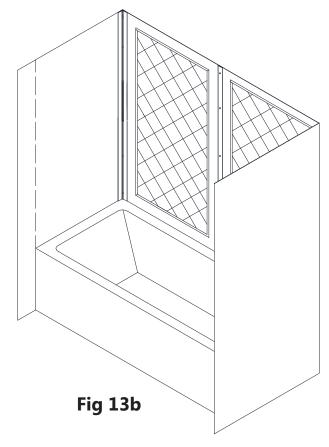
**Note:** Refer to the "D" dimension from **Step #3** to determine the finished cut size **"S"** for the **Side Panel (#02)** in the next steps. **(D - 1" = S)**
