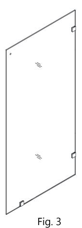
**3.** Place the **Return panel** (#22) on the preinstalled shower base or threshold. Position the panel up against the wall and level it vertically. Make sure the **Return panel** (#22) is aligned with the shower base or threshold and will create an opening that is **within the model dimensions** of the door section (<48" (SHEN-6134480) or <60" (SHEN-6134600) depending on the model size).
