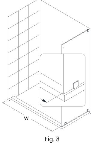
**9.** Your **Upper Guide rail (#03)** has been precut for your model width of: 48" or 60" (the actual rail is shorter than the model width by design).
