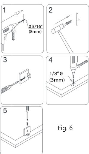
**7.** Place the **Return Panel (#22)** back in the designated position and assemble the Wall brackets (#19) to the Return Panel (#22).
