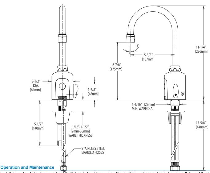
Installation should be in accordance with local plumbing codes. Flush all pipes thoroughly before installation. After installation, remove spout outlet or flow control flush acceptable of the control flush acceptable of th
