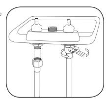
5 Attach handles and color-coded index buttons.
