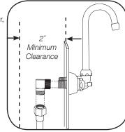
6 Follow instructions included with spout assembly. Attach spout and tighten.
