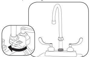
Remove outlet, flush lines for at least 2 minutes, and reinstall outlet.
