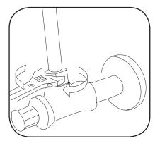
3 Attach water inlet hoses and tighten.
