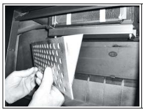
7. Once the combustor is installed completely so that all three tabs at touching the face of the dome, replace the flame shield. Note the brackets welded to the back flame shield are shaped like a triangle The point of the triangle should face down when installed correctly. Never operate your stove without the flame shield in place. The flame shield will protect the face of the combustor against damages from wood when loading and other possible damages that can occur during the cleaning process.
