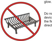
Do not use a grate or other device to elevate the fire off of the firebox floor. Burn the fire directly on the bricks.
