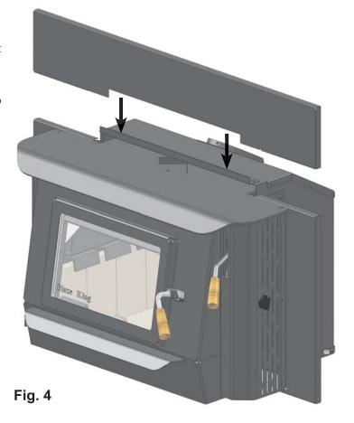
7. Hold the shroud top panel in place and slide the trim down over the shroud sides and top (see **Fig. 5**).
