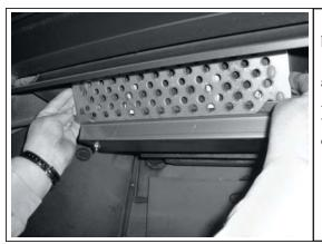
1. The removal of a Blaze King Catalytic combustor requires a small flat blade screwdriver or pocket knife. The stove fire must be out for at least 12 hours prior to the removal process. A combustor can reach 1400°F and hold high temperatures for several hours even after the fire is out. After waiting 12 hours, first remove the flame shield by simply lifting the shield off the two tabs at either side. Pay particular attention to orientation as there is a top and bottom edge to the flame shield.
