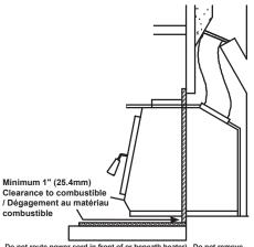
Electrical rating: (115 VAC, 60 Hz, 0.58 Amps. Risk of electrical shock. Disconnect power before servicing unit. Do not route power cord in front of or beneath heater). Do not remove bricks or mortar in masonry fireplace. Do not use grate or elevate fire. INSPECT AND CLEAN CHIMNEY FREQUENTLY.
