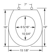
Ring thickness is 11/16" Ring thickness including the bumper is 1" Height of the seat with cover is 1-1/2"
