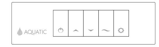
1 ON/OFF BLOWER 1<sup>st</sup> Press: The blower starts 2<sup>nd</sup> Press: The blower stops
