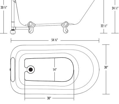
FEATURES Ibs (kg) Dimensional Tolerance ± 3/8". Dimensions needed for site preparation should be measured from the unit. Aquatic assumes no responsibility for preparatory work.
