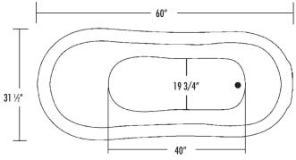
FEATURES Ibs (kg) Dimensional Tolerance  $\pm$  3/8". Dimensions needed for site preparation should be measured from the unit. Aquatic assumes no responsibility for preparatory work.
