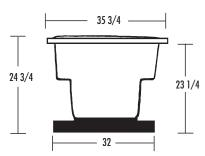
FEATURES Ibs (kg) Dimensional Tolerance ± 3/8". Dimensions needed for site preparation should be measured from the unit. Aquatic assumes no responsibility for preparatory work.
