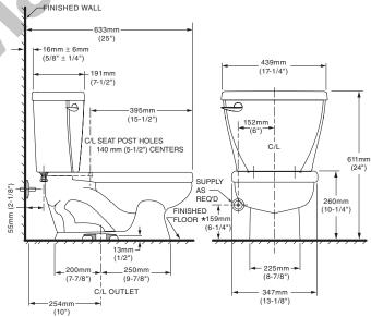
NOTES: THIS COMBINATION IS DESIGNED TO ROUGH-IN AT A MINIMUM DIMENSION OF 254mm (10) FROM FINISHED WALL TO C/L OF OUTLET \* DIMENSION SHOWN FOR LOCATION OF SUPPLY IS SUGGESTED. SUPPLY NOT INCLUDED AND MUST BE ORDERED SEPARATELY.
