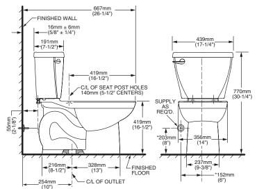
NOTES: THIS TOILET IS DESIGNED TO ROUGH-IN AT A MINIMUM DIMENSION OF 254MM (10") FROM FINISHED WALL TO C/L OF OUTLET SUPPLY NOT INCLUDED WITH FIXTURE AND MUST BE ORDERED SEPARATELY.
